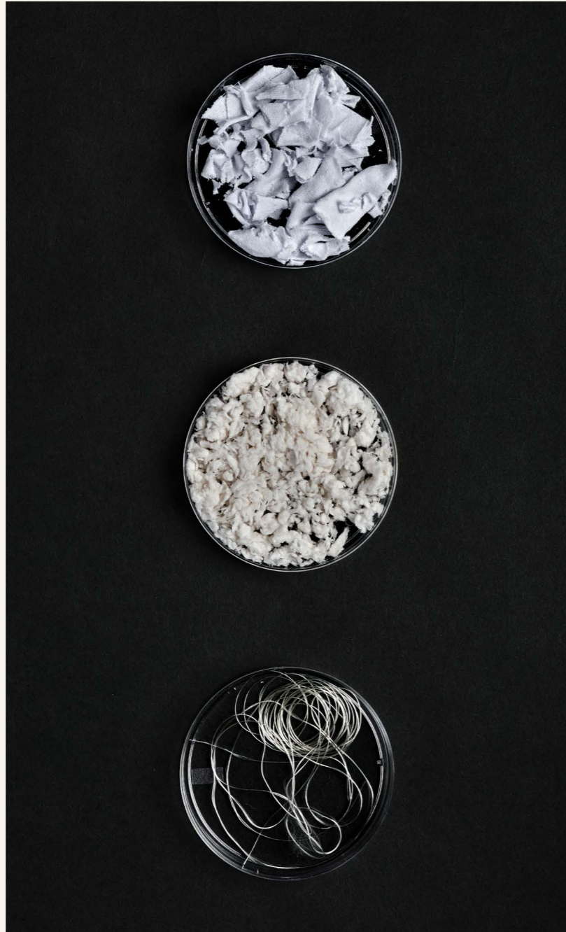
Circ's hydrothermal process turns polyester-cotton blend fabrics (left) into cellulose (center) and recycled polyester (right). Source: Circ
