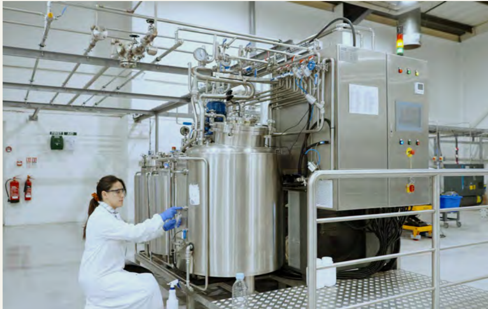
Colorifix growing engineered microbes in their fermentor with renewable feedstocks. The microbes divide every 20 minutes and results in a large quantity of dye liquor within one to two days
